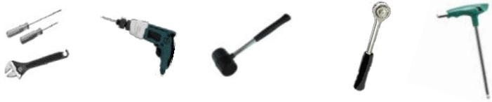
Installation tools: screwdriver, wrench ,Φ10 drill, hammer, socket wrench set and Hexagon keys.
