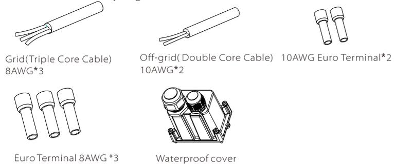
Step 2: The Grid and Off-grid cables go through the corresponding Grid and Off-grid ports of the waterproof cover.
