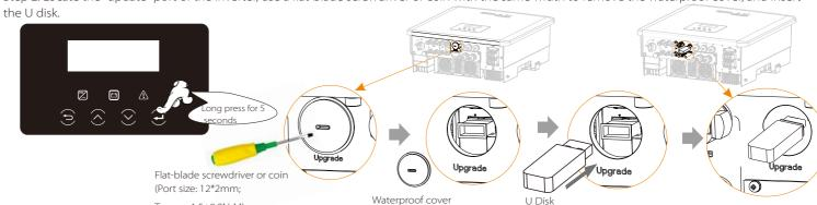
Step 3. LCD operation, enter the upgrade interface "update", as shown below(a): Please press the up and down keys to select ARM, then press the bottom of the page to select "OK", press the enter key to enter the software version interface;
