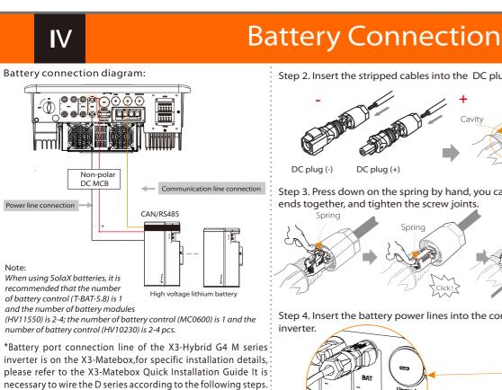
Step 1. Prepare 8 AWG battery power line, find the DC
