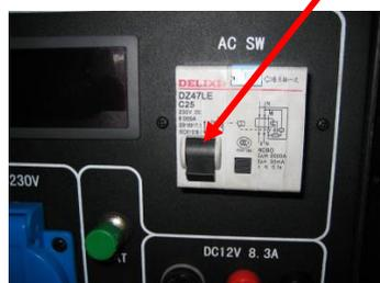
DES QUE VOTRE MACHINE FONCTIONNE L'ECRAN DIGITAL VOUS INDIQUERA A LA SUITE ET EN BOUCLE, LA TENSION, LA FREQUENCE ET LE NOMBRE D'HEURES DE FONCTIONNEMENT
